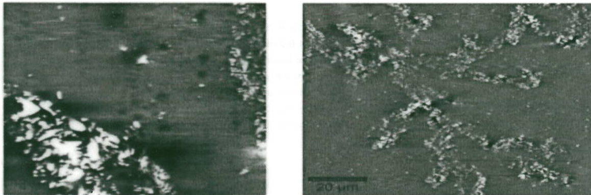
Figure 9. AFM Topography for AC-30 Modified with Banana Bags
