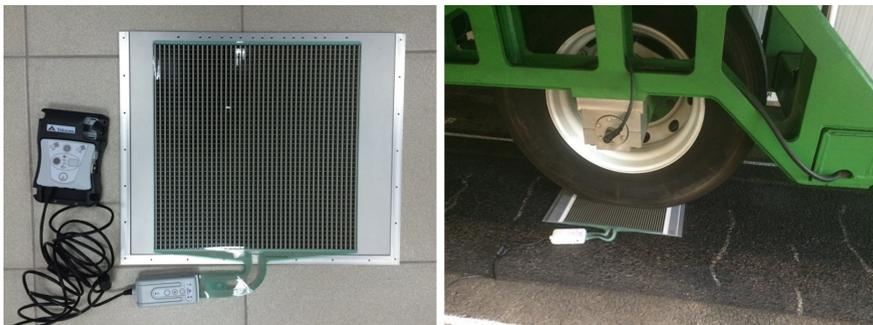
Fig. 2 Tire footprint acquisition system
