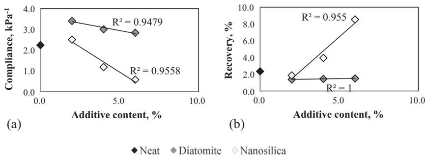
Fig. 7. Influence of additive content on a) compliance and b) elastic recovery of asphalt binders.
