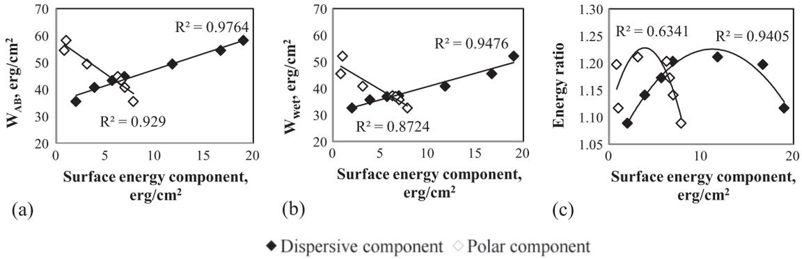
Fig. 5. Influence of surface energy components of binder on a) work of adhesion, b) work of debonding and c) energy ratio.
