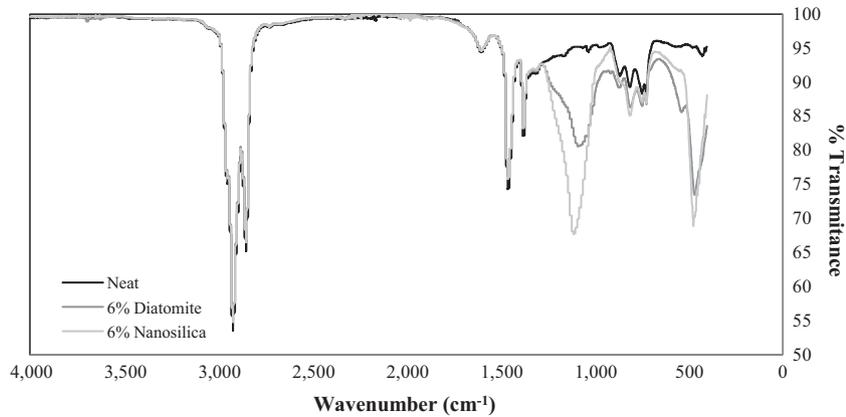
Fig. 1. Infrared spectra of 6% diatomite and 6% nanosilica modified binders. The spectra of neat binder is shown for comparison.
