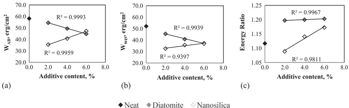
Fig. 4. Influence of additive content on a) work of adhesion, b) work of debonding and c) Energy Ratio of the binder-limestone combinations.
