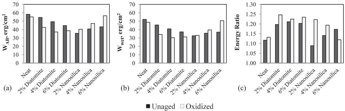
Fig. 6. Effect additives on a) work of adhesion, b) work of debonding, and c) energy ratio of unaged and oxidized binders.
