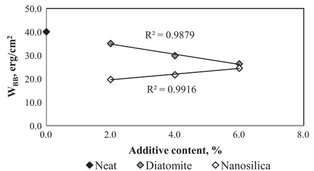
Fig. 2. Influence of additive content on the cohesion of unaged asphalt binders.
