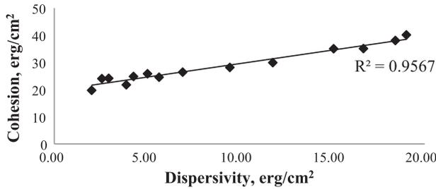
Fig. 3. Cohesion as a function of dispersivity of asphalt binders.
