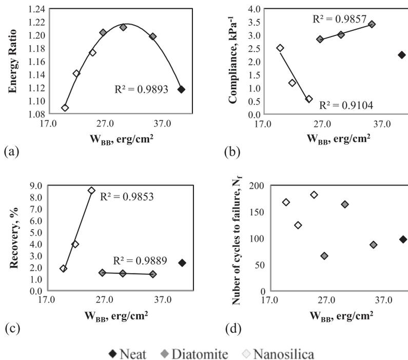
Fig. 9. Relationship between cohesion of the binders and a) energy ratio, b) compliance, c) elastic recovery and d) fatigue.
