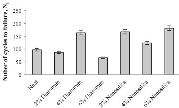
Fig. 8. Number of cycles to failure for neat and modified binders.
