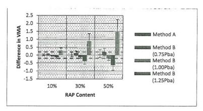
Figure 11. Difference in VMA versus RAP content based on centrifuge (error bars represent minimum and maximum difference in VMA.)
