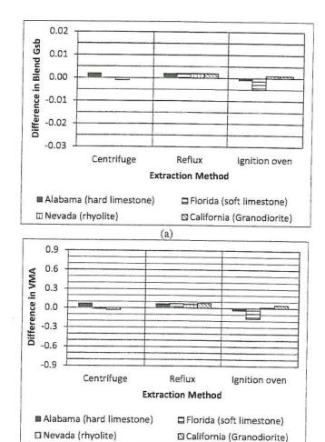
Figure 2. (a) Difference in blend  $G_{sb}$  and (b) VMA for 10% RAP content, Method A.
