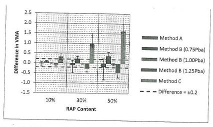
Figure 13. Difference in VMA versus RAP content based on ignition oven (error bars represent minimum and maximum difference in VMA).
