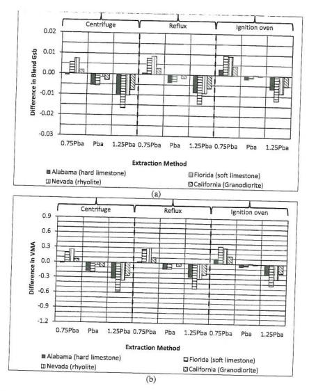
Figure 6. (a) Difference in blend  $G_{sb}$  and (b) VMA for 30% RAP content, Method B.
