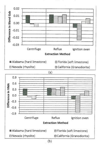
Figure 4. (a) Difference in blend Gst and (b) VMA for 50% RAP content, Method A.
