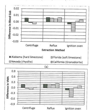
Figure 3. (a) Difference in blend  $G_{sb}$  and (b) VMA for 30% RAP content, Method A.
