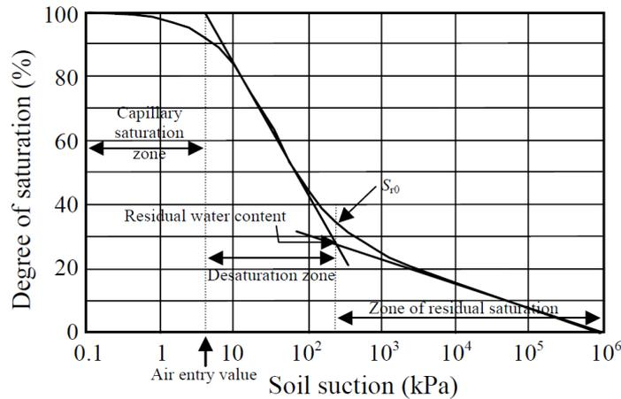
**Figure 2. Soil-water characteristic curve showing the regions of de-saturation (Sillers et al, 2001)**
