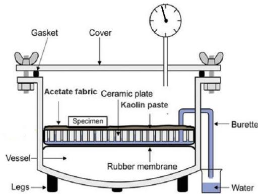
**Figure 5. Pressure Plate Test Apparatus (ASTM C1699-09)**
