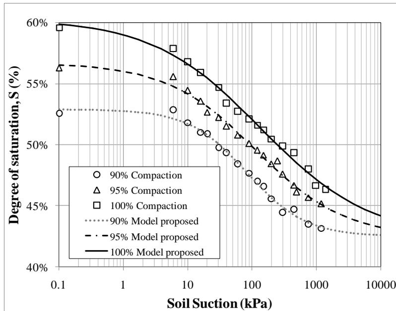
Figures 8. Soil-water characteristic curves model fitted to the experimental data
