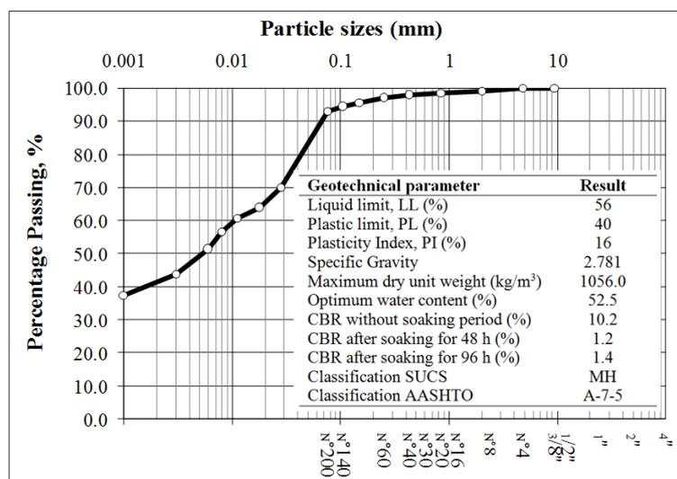
**Figure 4. Geotechnical characterization and particle size distribution**
