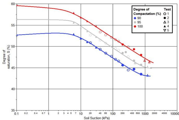
**Figure 6. Soil water characteristic curves of soil studied by different degree of compaction**
