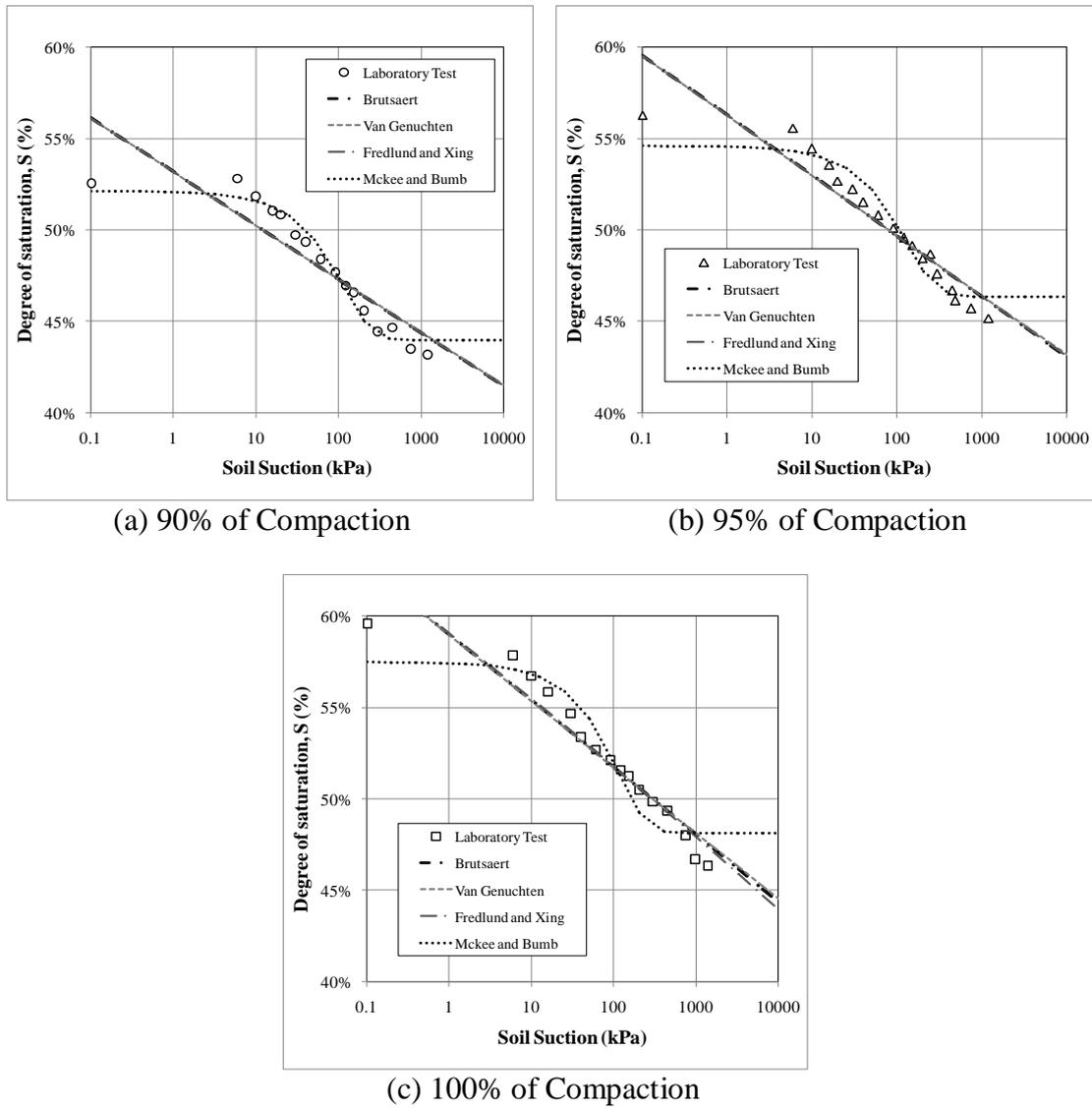
**Figures 7. Soil-water characteristic curves model for the laboratory test results**
