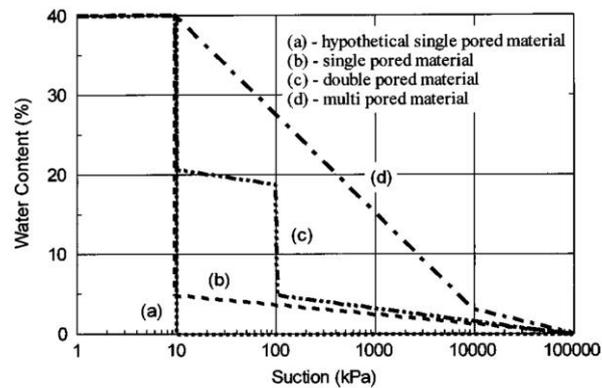
**Figure 3. General shape of soil-water characteristic curve according to pore size distribution (Marinho, 2005)**
