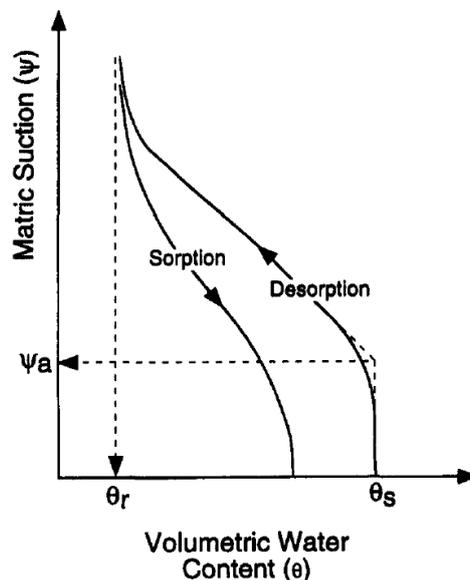
**Figure 1. Typical Soil-Water Characteristic Curves for Desorption and Sorption (Zhou et al., 2012)**
