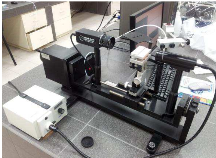
FIGURE 2 Goniometer used in Contact Angle Measurements
