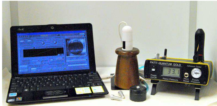
FIGURE 1 PATTI Testing Equipment (Source: http://www.semico.org )
