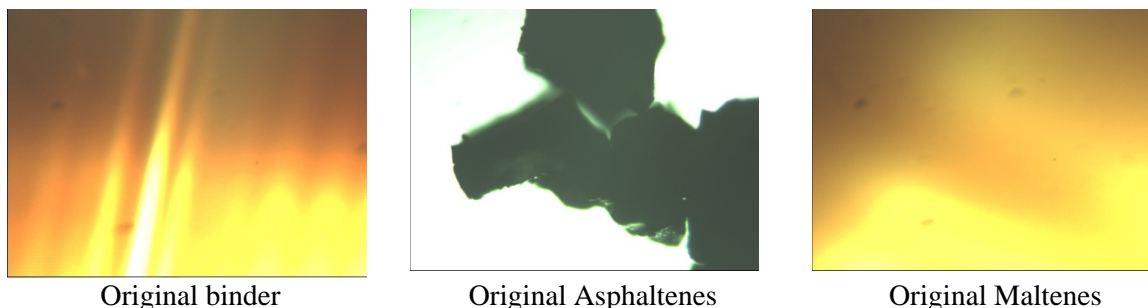
FIGURE 2 Polarized light microscopy analysis of original (unaged) samples
