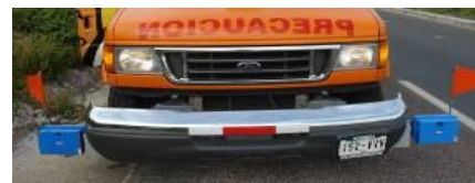
(c) Profilometer for IRI survey
