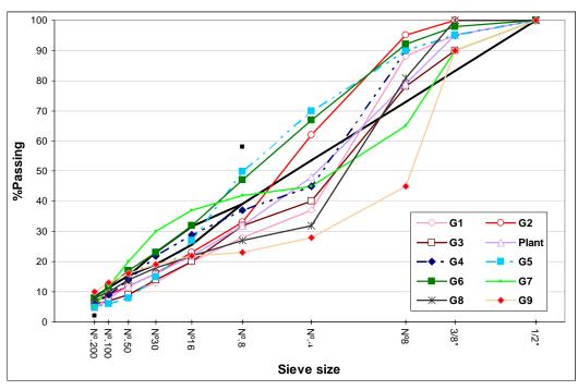
FIGURE 2 Aggregate Gradations Used in the Study
