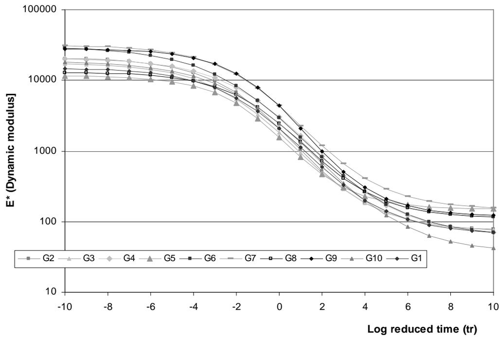
295 **FIGURE 3 Master Curves of Dyanmic Modulus fir the Various Gradations Used in the**
