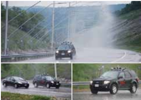
The ByWire XGV is being used as the mobile robotics research platform for testing the Long Range Obstacle Detection cross-platform software and sensor payload, which will enable high-speed autonomous vehicle operations up to 100 KPH.
