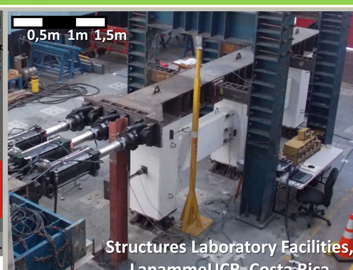
Global rocking mechanism: (i) Hybrid joint with unbonded post-tension and mild-steel reinforcement / (ii) Partially restrained (PR) connection
