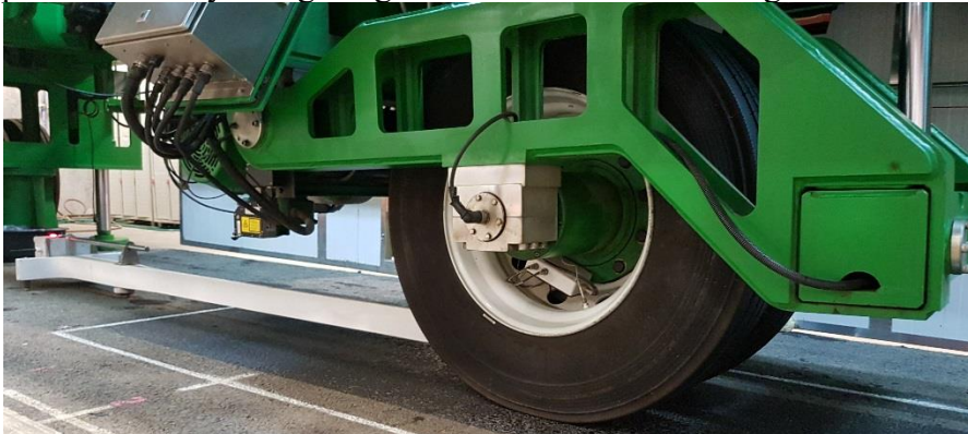
4 5 FIGURE 4 Measurements with RSD equipment and HVS tire. 6
