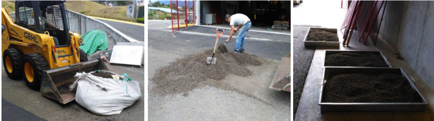
Figure 12. RAP handling in the laboratory.
